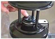
Assemble Clamp Plate onto Thread
