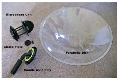
Major components of the parabolic microphone.
